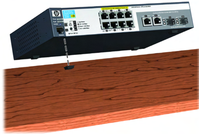
Figure 2-9. Horizontal Surface Mounting
